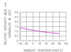
Fig.4 RELATIVE INTENSITY VS. TEMPERATURE
