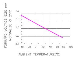
Fig.3 FORWARD VOLTAGE VS. TEMPERATURE
