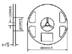
Dimensions of Tape (Unit: mm)
